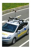
The IP-S2 standard system includes three high-resolution LiDAR scanners that cover the vehicle path at ground level and sweep the adjacent areas to a distance of 30 meters.
